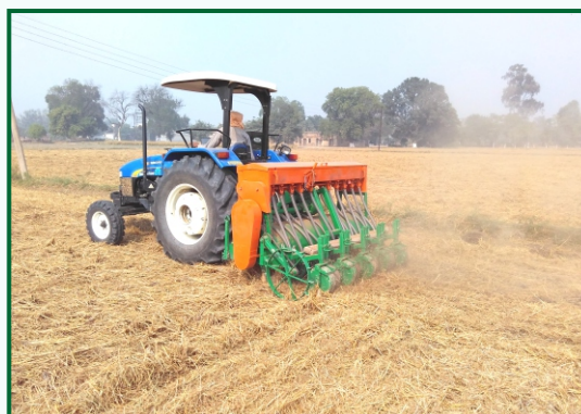
Wheat sowing with Happy Seeder for paddy straw management
